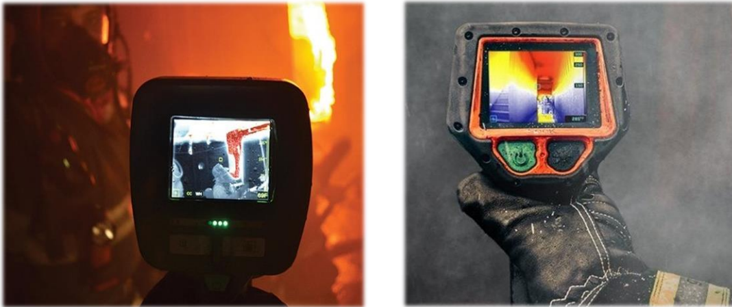
The images show a third generation TIC (10 years+) on the left and a new fifth generation TIC (new) on the right.
