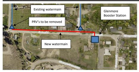
A recent analysis of the distribution system identified that the two pressure regulating stations can be effectively removed if water is supplied from the Glenmore Road pressure zone. Removal of these two stations will reduce operational costs, eliminate future replacement costs, and eliminate a confined space hazard.
