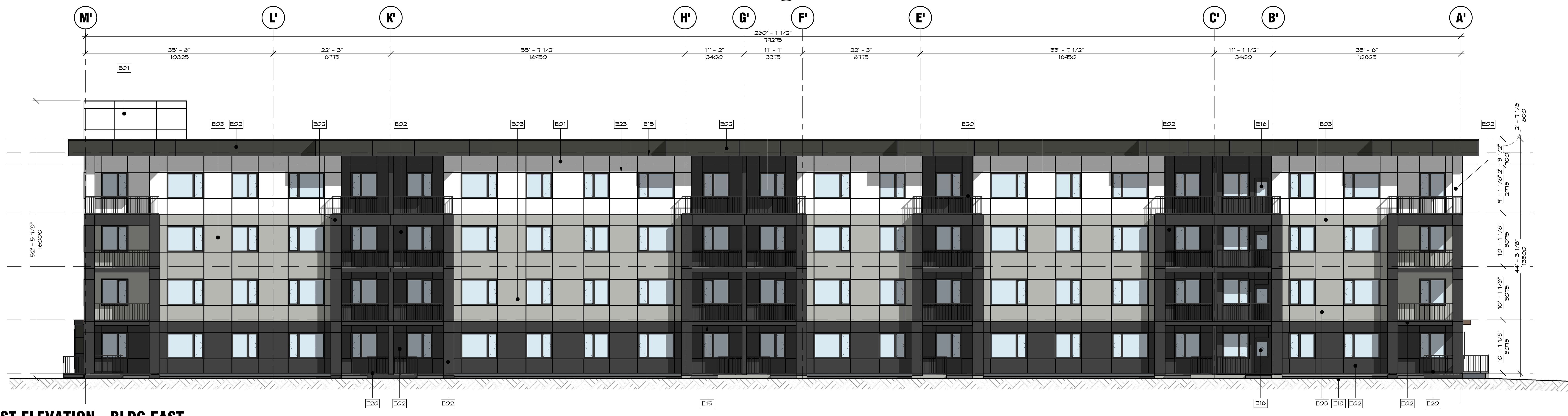
A1 EAST ELEVATION - BLDG EAST DP301 SCALE #1: 100
