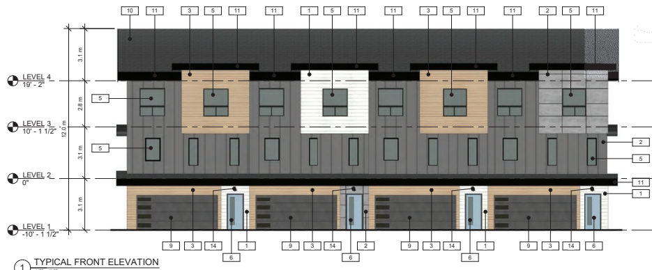
1 TYPICAL FRONT ELEVATION 1/8" = 1'-0"
