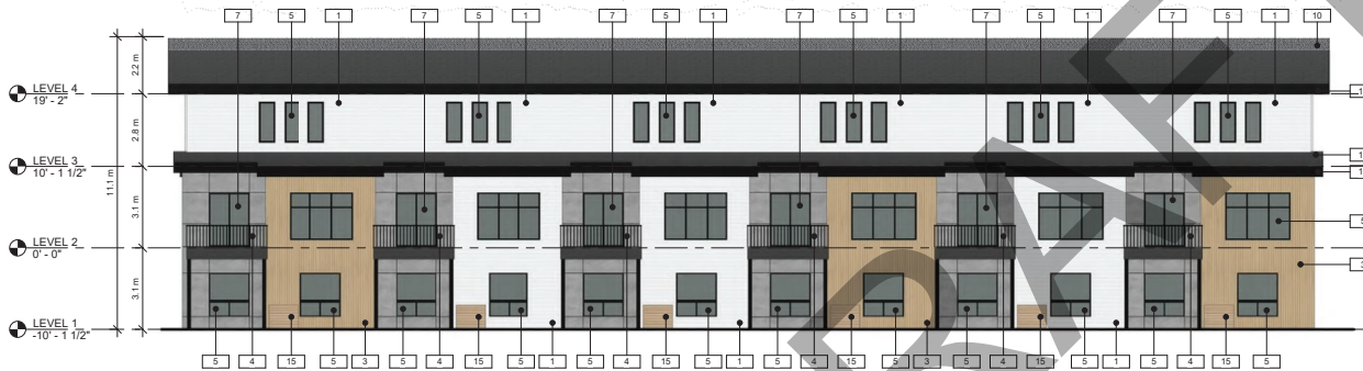
2 TYPICAL SOUTH ELEVATION 1/8" = 1'-0"
