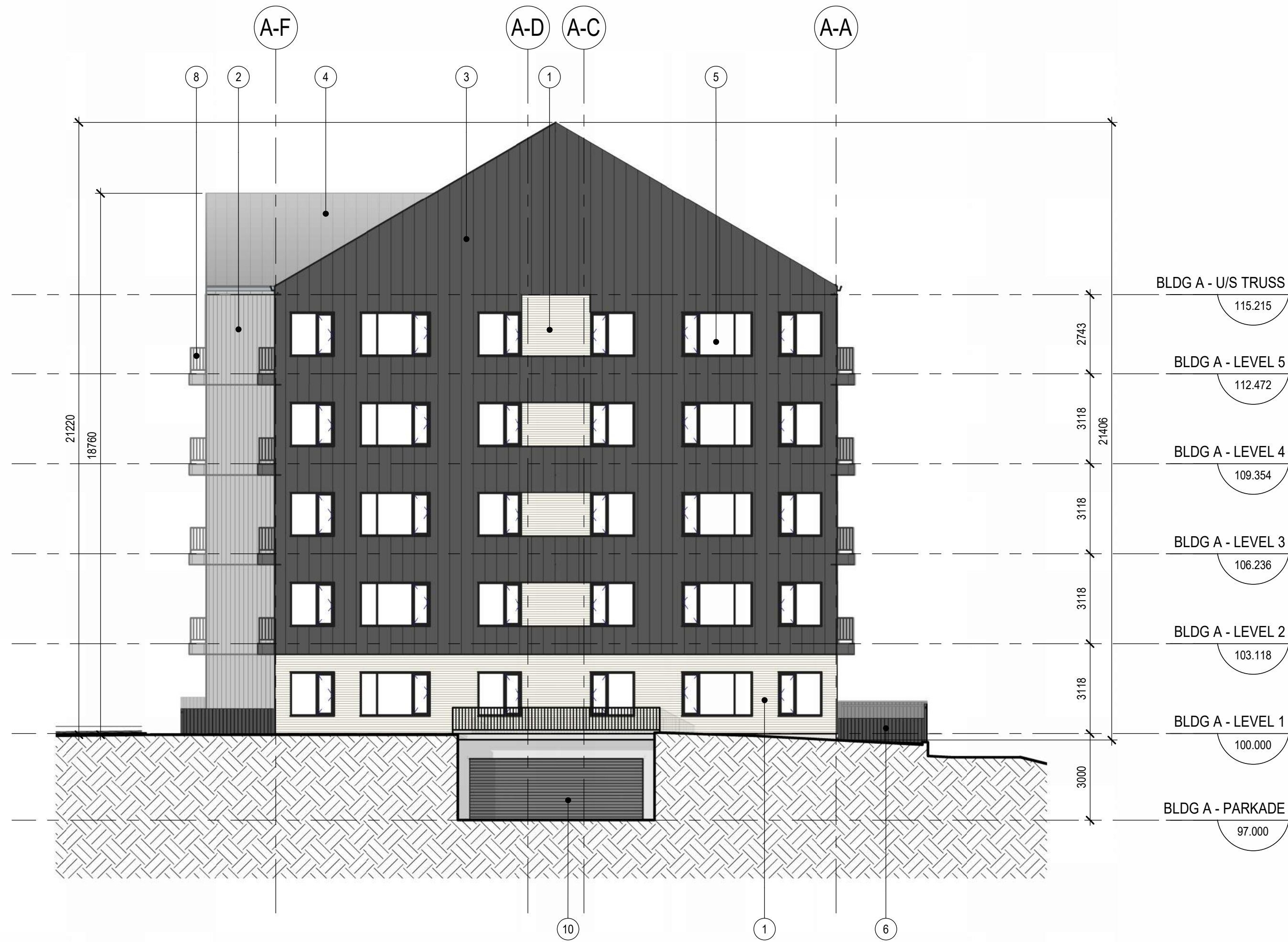
2 EAST ELEVATION - BUILDING A DP3.1 SCALE: 1 : 125
